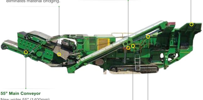
New wider 55" (1400mm) main conveyor, giving large stockpile capacity. Conveyor lowers and raises hydraulically.
