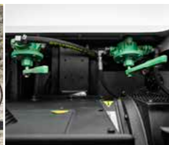
Oil sump pump and containment pump
